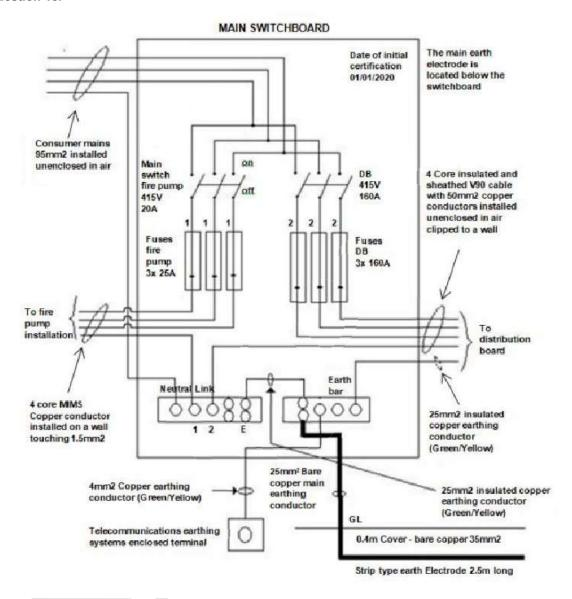
The drawing above shows the MAIN SWITCHBOARD of an industrial installation originating at the consumer's mains and contains contraventions to the Wiring Rules.
