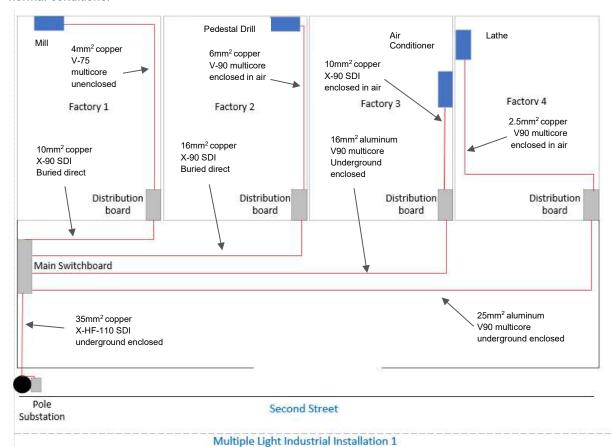
Client: Darren Wall Location Cable **Distance** Maximum Voltage **Demand** Drawing title: Site plan Main Switchboard **Consumer Mains** 11m 130A 400/230V Date: 5 November 2024 Factory 1 Distribution board Sub Mains 14m 57A 400/230V Location: 65 Imagine Sub Mains 48A 400/230V Factory 2 Distribution board 22m St, Carlton Factory 3 Distribution board Sub Mains 34m 60A 400/230V 55A 400/230V Factory 4 Distribution board Sub Mains 50m
