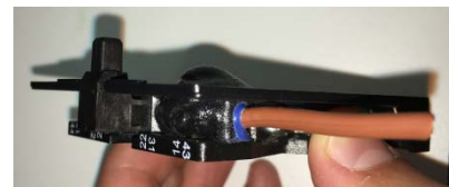
Failed contactor from Inverter
