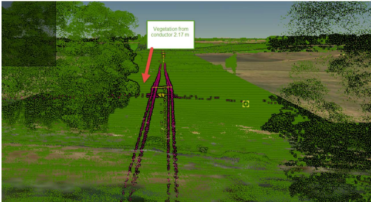
Figure 7: LiDAR image of site provided by Powercor
