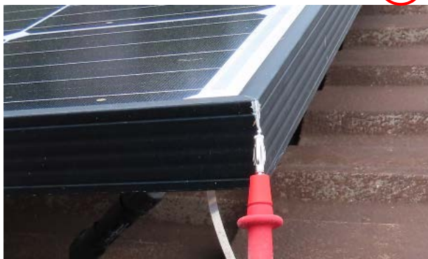
Image above showing earthing points at the rear of a Hanwha Q Cells PV Module .
